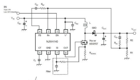
8| NJW4140 in non-isolated boost converter circuit
