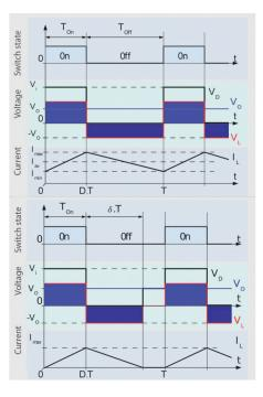
2| Continuous and discontinuous step down converters
