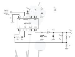
6 NJW4152 buck converter reference circuit
